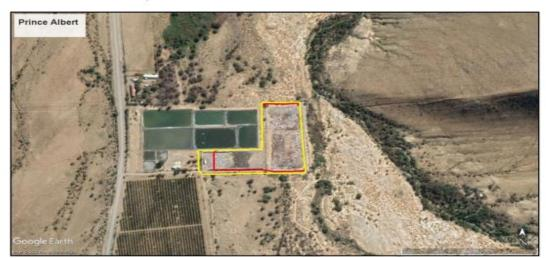
The permit restricts the maximum height of the site to 2m above ground level. The remaining airspace on the used footprint up to a height of 2m and 1:4 side slopes, calculated using the June 2022 topographical survey, is approximately 5, 313m<sup>3</sup>.
