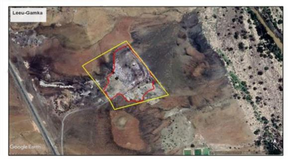
This site has been issued with an operational licence, also without specifying a maximum allowed height. Reshaping and compacting was done in order to increase remaining operational lifetime.
