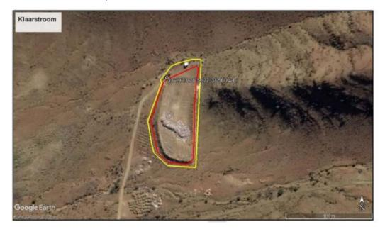
Based on the used footprint, 1:4 side slopes and a height of 3m at the southern edge, the available airspace was calculated as 3, 877m<sup>3</sup> with use of the topographical survey of June 2022.
