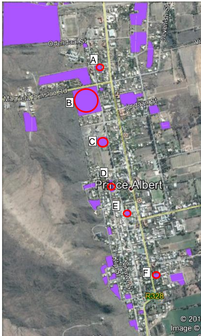
Figure 7.5: Candidate Sites for Stormwater Detention Ponds in Prince Albert South
