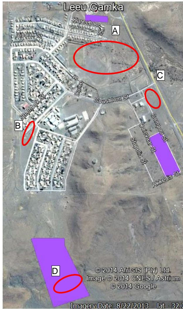
Figure 7.7: Candidate Sites for Stormwater Detention Ponds in Leeu Gamka
