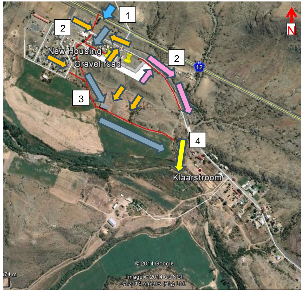
Map 4.4: Klaarstroom Existing Stormwater System and Drainage Paths
